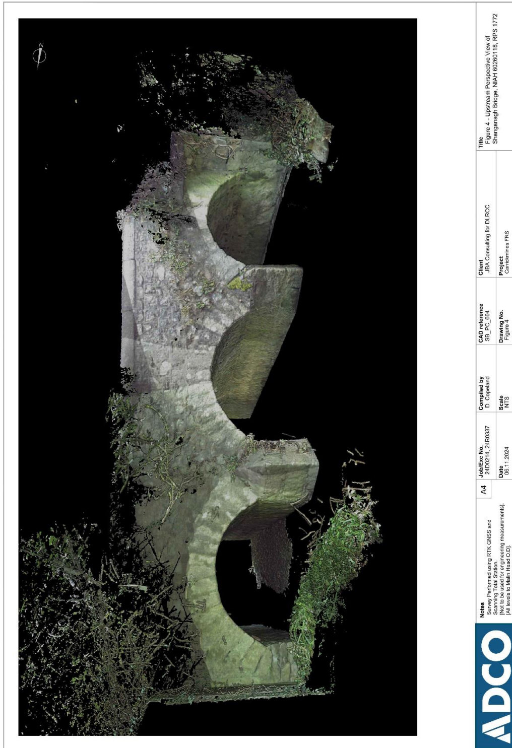
Figure 4: Point Cloud image derived from laser scan survey of Shanganagh Bridge. View looking downstream towards bridge.
