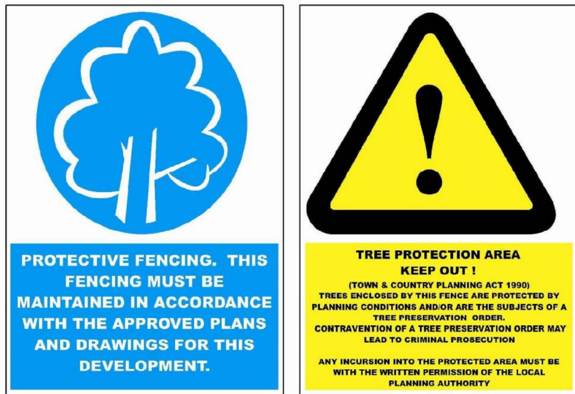
Figure 6-6 Example warning signage to be placed on protective fencing
